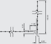
Renderplas PVC reveal head beads with drip detail and glass fibre reinforcement mesh. Designed for function and speed of installation at the head of all EWI and thin coat rendered reveals
